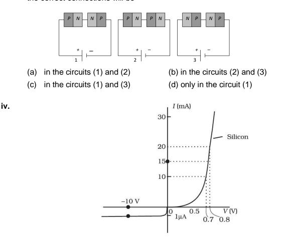
The V-I characteristic of a diode is shown in the figure. The ratio of the resistance of the diode at I = 15 mA to the resistance at V = -10 V is (a) 100 (b)  $10^{6}$  (c) 10 (d)  $10^{-6}$
