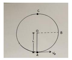
Derive an expression for minimum velocity at point A so that it reaches point C. Also calculate its magnitude.
